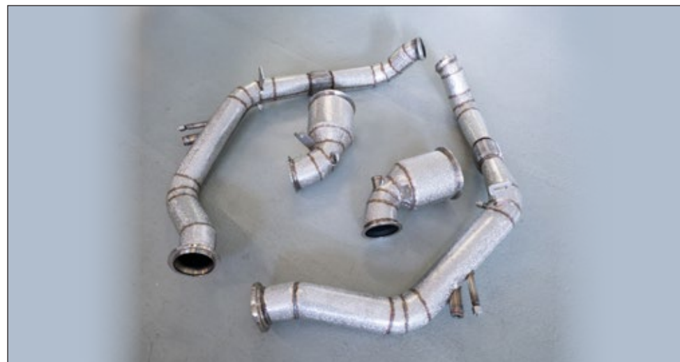
Down pipe with EUR6 with Cat 200 Cell - V8
