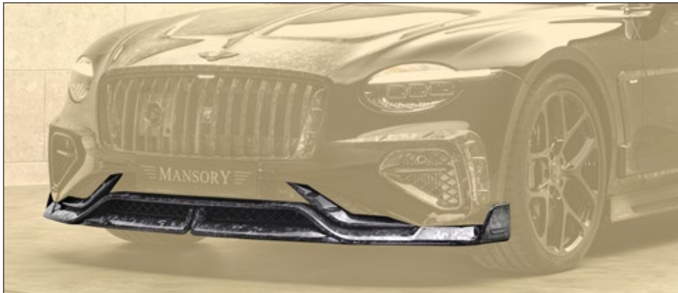
Front lip visible carbon fibre without clear coat
