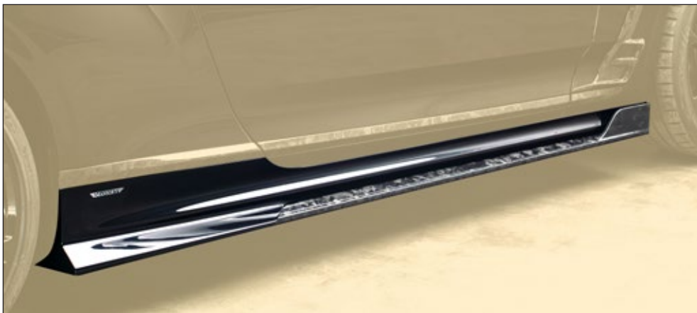
Side skirts 2 parts set - left & right ( with chrom skirt bar ) side skirts lip visible carbon fibre without clear coat
