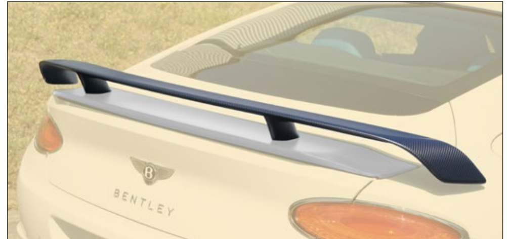
Biplane performance wing - visible carbon
