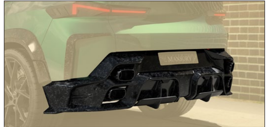
Rear diffuser visible carbon fibre without clear coat with double exhausts blinds
