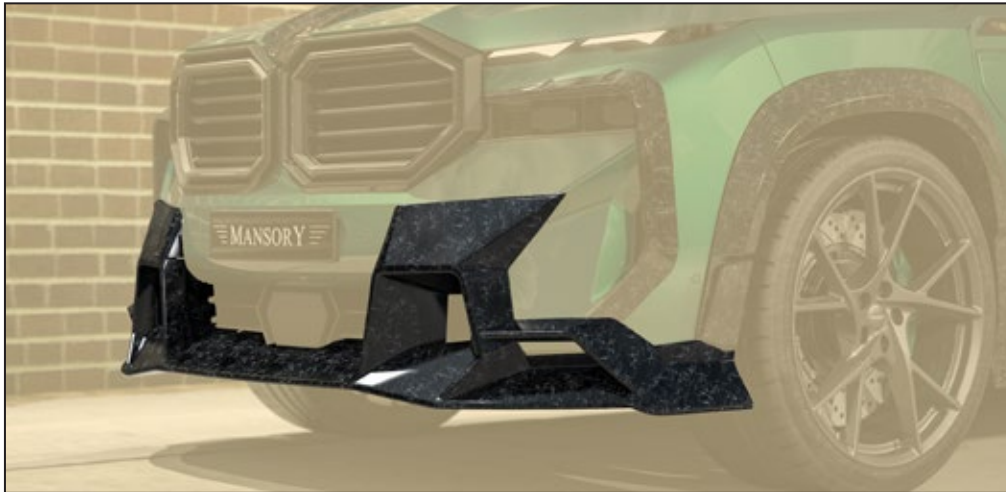
Front lip visible carbon fibre without clear coat
